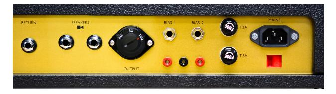
DUAL BIAS on the back panel allows you to set the bias of output tubes. It is currently set to 32mV per tube. Use a Digital Multimeter. When changing tubes, always start by turning the BIAS 1 and BIAS 2 pots fully counter-clockwise, a speaker load connected, and MVC set to zero. As you turn the BIAS 1 and BIAS 2 pots SLOWLY clockwise, the tubes with starting drawing current. Jump back and forth between the two output tubes and bring them up together.
