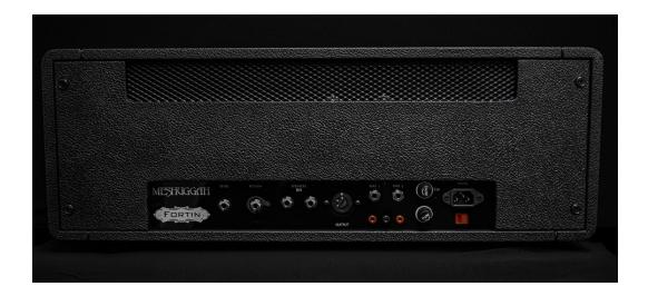
DUAL BIAS on the back panel allows you to set the bias of output tubes. It is currently set to 32mV per tube. Use a Digital Multimeter. When changing tubes, always start by turning the BIAS 1 and BIAS 2 pots fully counter-clockwise, a speaker load connected, and MVC set to zero. As you turn the BIAS 1 and BIAS 2 pots SLOWLY clockwise, the tubes with starting drawing current. Jump back and forth between the two output tubes and bring them up together.
