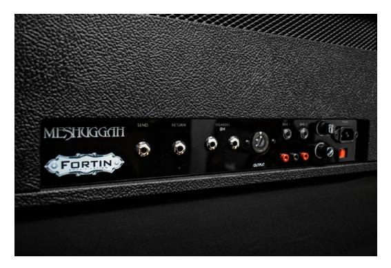
FX LOOP is a passive series insert loop. When not used it is exactly as the amps I made for Meshuggah since those did not have loops in them. Here you can insert effects but keep in mind that the signal level out of the SEND will change because the MVC is before the tone stack and loop.
